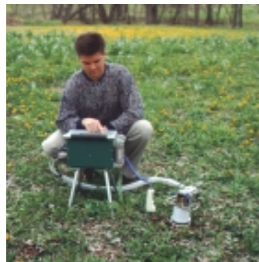
The LI-6400 console displays flux rate calculations in numeric and graphical form for evaluation in the field.
