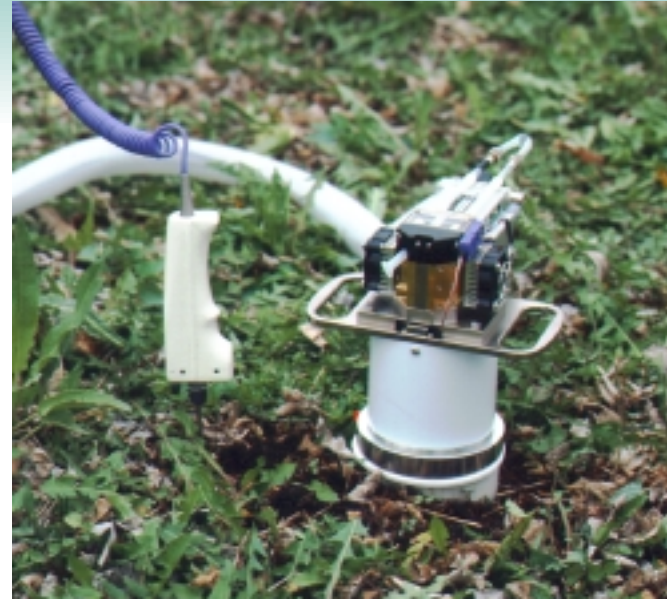
Figure 1. The CO 2 and H 2 O analyzers in the LI-6400 sensor head are connected directly to the soil chamber for fast response.
