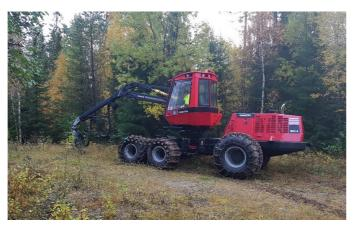
In the field trials, we used a Komatsu 901.4 harvester purchased by Swedish Smallwood project partners. The machine weighs about 16 tons, has a reach of 11 m and is 270 cm wide. It is equipped with a special accumulating felling head made by Swedish manufacturer Bracke C16.c, which collects bunches of thin trees. The accumulating felling head can be very effective in suitable stands. The advantages of this accumulating felling head are its robust construction and easy maintenance.
