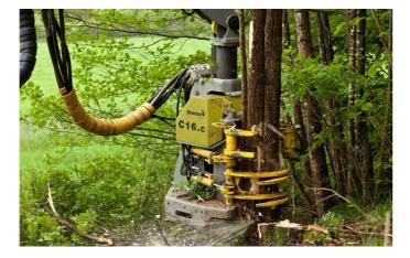
We used Bracke C16.c accumulating felling head in the field trials, but this is not the only processor head of this type on the market.
